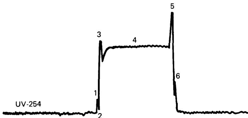
Fig. 5. Isotachopherogram resulting from a 7.5 nanomole injection of CP Lot EL58633. Zones: 1 = electrolyte contaminant; 2 = non-UV-absorbing unknown; 3 = amidine ( 0.5 \pm 0.02\% ); 4 = CP ( 95.6 \pm 0.3\% ); 5 = amide ( 3.9 \pm 0.04\% ); 6 = UV-absorbing unknown. Percentages were calculated from relative areas, with uncertainties at the 95% confidence level based on three replicates.
